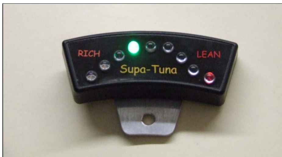
Picture 4 With this LED illuminated, it is starting to get close to the ideal tune.
